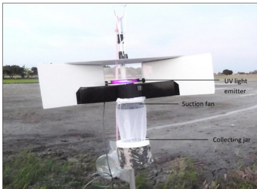
Figure 1. A close up of an ultraviolet (UV) suction blacklight trap placed in the rice field.
