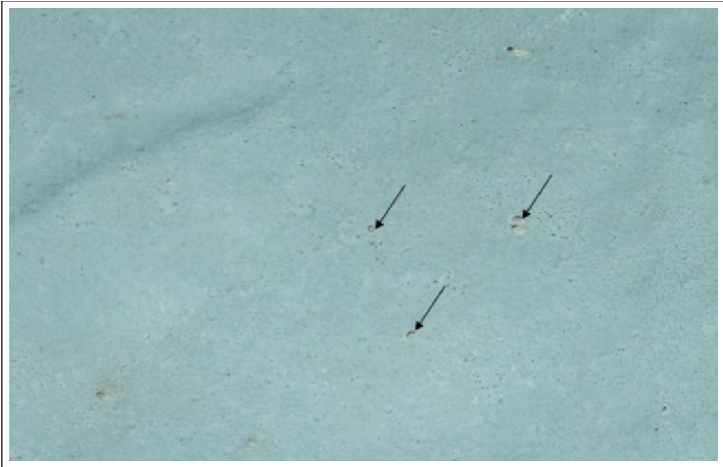
Figure 1. Hide of bovine showing marked ticks bite lesions with small pin point pores after pickling and bluing process of leather tanning process.
