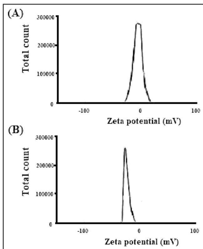
**Figure 3.** The results of the zeta potential of the zinc oxide nanoparticles (A) and linalool-zinc oxide nanoparticles (B).
