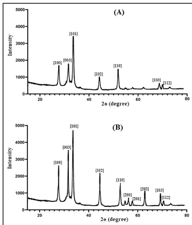
**Figure 2.** The X-ray diffraction analysis of the zinc oxide nanoparticles (A) and linalool-zinc oxide nanoparticles (B).
