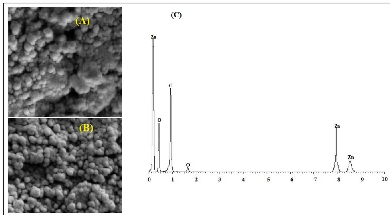
**Figure 1.** scanning electron microscope of zinc oxide nanoparticles (A) and linalool-zinc oxide nanoparticles (B, Lin-ZNP) as well as energy dispersive X-ray (C, EDX) analysis of Lin-ZNP.
