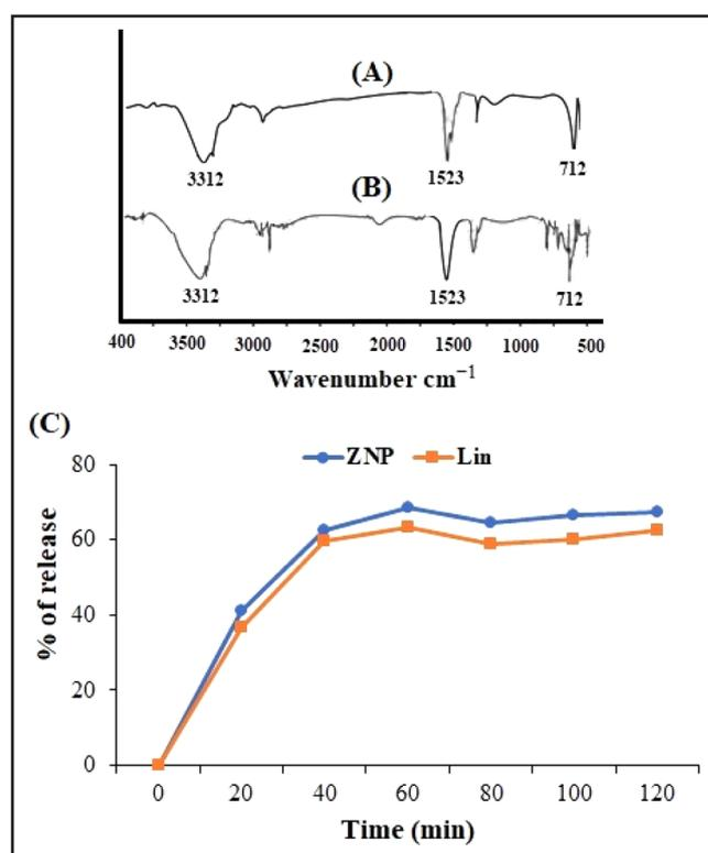
**Figure 4.** The Fourier transform infrared spectroscopy of the zinc oxide nanoparticles (A, ZN) and linalool-zinc oxide nanoparticles (B) and the release kinetics of linalool and ZN (C).
